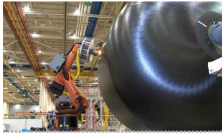
Composite liquid- hydrogen fuel tanks
